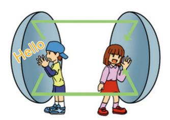
be collected all in one point. On the other hand, the sound that was made from a focus position to paraboloid surface reflects by the paraboloid surface and travels parallel in an axial direction. Thus, it is possible to collect sound and electric waves that spread all around and deliver them in one place. Therefore, parabola is used for receiving antennas of satellite broadcasting and international transmitters and receivers.
