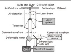
How to Reduce the Effect of Scintillation
