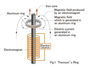
By pressing the button, the aluminum ring jumps high. Because there is no spring or launcher, it seems that the ring jumps suddenly by some invisible force. This invisible force was created by the coil beneath the ring. When electricity suddenly flows through the coil, the
