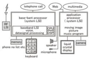
Fig. System of mobile phone
