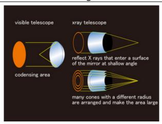
How does an X-ray telescope work?
